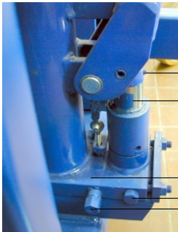
Bleeder screw Pump piston Valve block High-pressure valve core Low-pressure valve core
